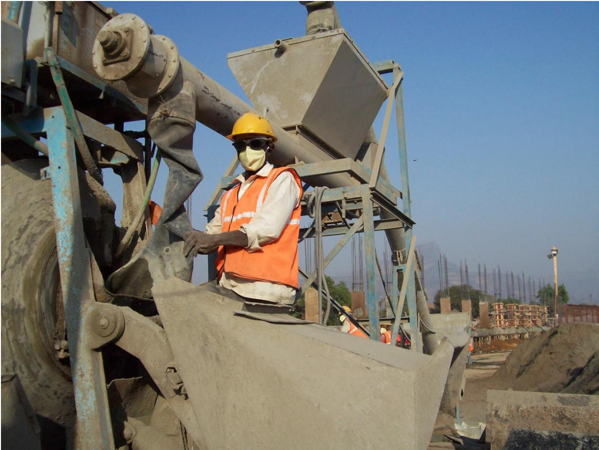
BATCHING PLANT OPERATION WITH SAFE WORKING PRACTICE BY USING PROPER PPE
